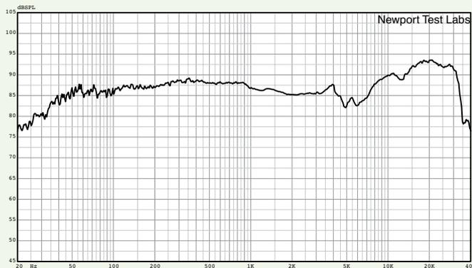
**Graph 5:** Frequency response. Trace below 800Hz is the averaged result of nine individual frequency sweeps measured at three metres, with the central grid point on-axis with the tweeter using pink noise test stimulus with capture unsmoothed. This has been manually spliced (at 800Hz) to the gated high-frequency response from Graph 2.
