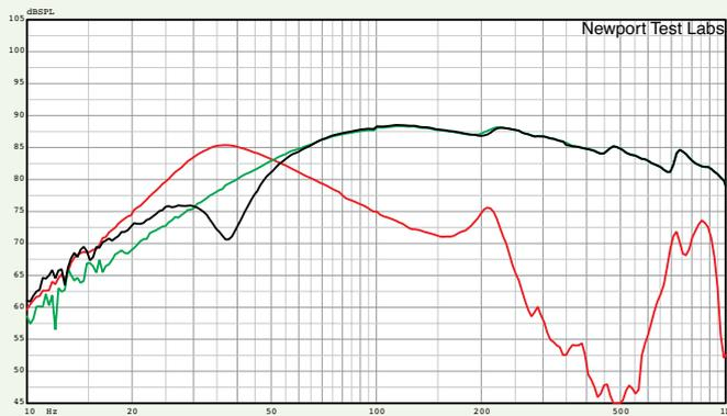
**Graph 3:** Low frequency response of front-firing bass reflex port (red trace) and woofer with open bass reflex port (black) and with port blocked (green trace). Nearfield acquisition. Port/woofer levels not compensated for differences in radiating areas.
