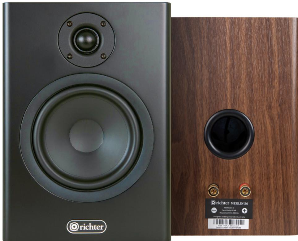
Also new is the shape of the bass reflex port which exits just below the centre of the rear; this flares from a diameter of 35mm at its inlet inside the cabinet to a diameter of 50mm at the flared exit, over a 100mm length.
