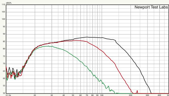
**Graph 5.** Nearfield response of bass driver with both ports plugged. Black trace is with low pass filter set to maximum (160Hz), red trace is with low pass filter set to 70Hz, green trace is with low pass filter set to minimum (40Hz). [Richter 10.6 Subwoofer.]
