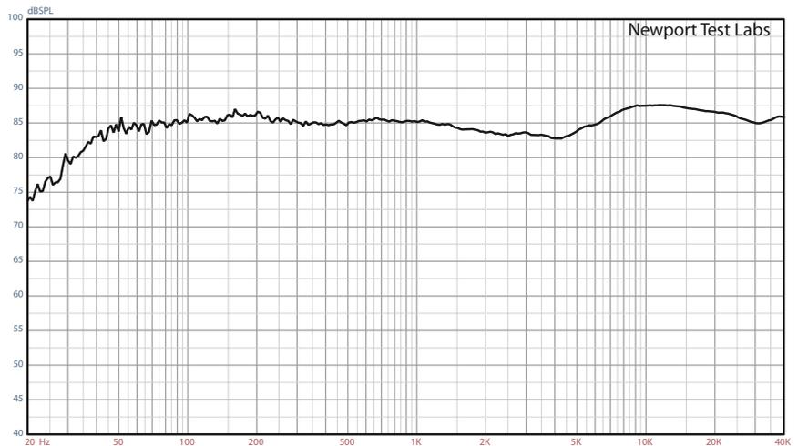
Graph 1. Averaged in-room frequency response using pink noise test stimulus. Trace is the averaged result of nine individual frequency sweeps measured at three metres, with the central grid point on-axis with the tweeter. [Richter Wizard V Loudspeaker]
