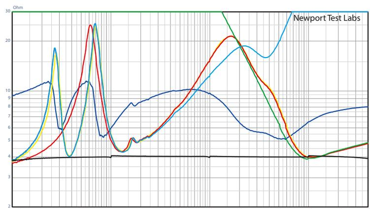
Graph 4. Impedance modulus of left (red trace) and right (yellow trace) speakers plus phase (dark blue trace), high-pass section (green trace, and low-pass section (light blue trace). Black trace is reference 4 ohm precision calibration resistor. [Richter Wizard V]
