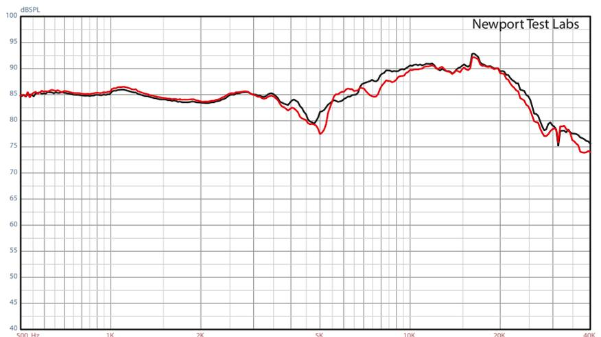
Graph 2. High-frequency response, expanded view, showing difference in response between grille on (red trace) and grille off (black trace). Test stimulus gated sine. Microphone placed at three metres on-axis with dome tweeter. [Richter Wizard V Spkrs]
