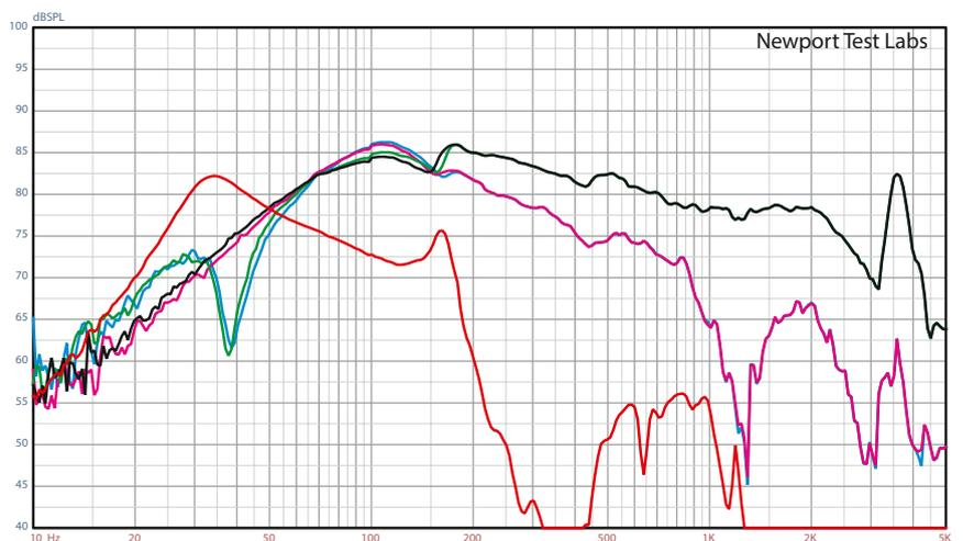
Graph 3. Low frequency response of rear-firing bass reflex port (red trace), upper bass/midrange driver without bung (green trace) and with bung (black trace) and lower midrange driver without bung (blue trace) and with bung (pink trace). Nearfield acquisition. Port/woofer levels not compensated for differences in radiating areas. [Richter Wizard V]
