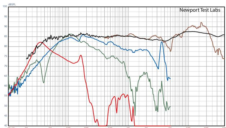
Graph 5. Composite response plot. Red trace is output of bass reflex port. Dark blue trace is anechoic response of upper driver with port bung fitted. Green trace is anechoic response of lower driver without port bung. Brown trace is gated (simulated anechoic) response above 400Hz. Black trace is averaged in-room pink noise response. [Wizard V]
